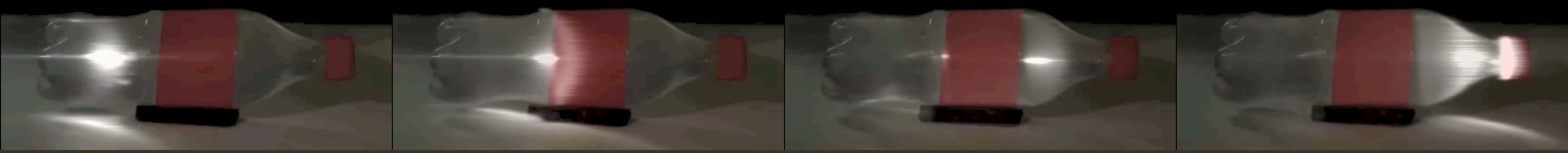
Pulse of light going through a bottle at one trillion frames per second (Camera Culture Group, MIT Media Lab)
